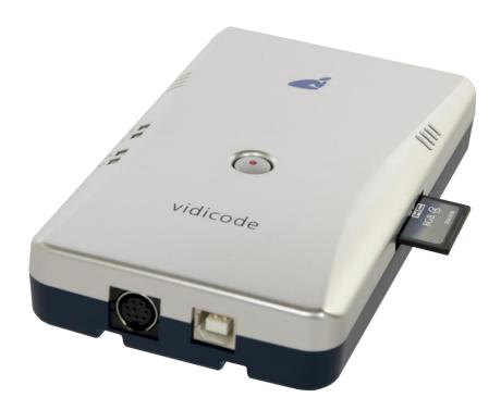
The V-Tap Analog is a device that can record the audio from an analog telephone line or any telephone that works with a handset. The captured data is stored onto an SD card and can optionally be sent to an external server (an Apresa recorder or the V-Archive software running on a PC).
