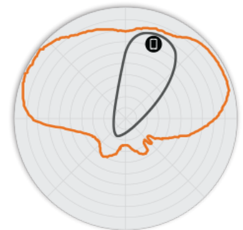
Figure 5. R710 5GHz Elevation Antenna Patterns
