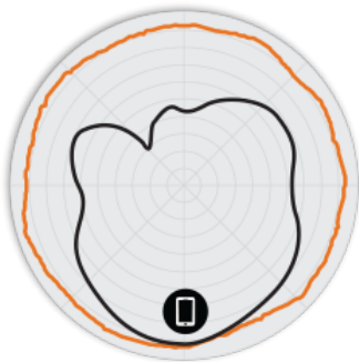
Figure 2. R710 2.4GHz Azimuth Antenna Patterns
