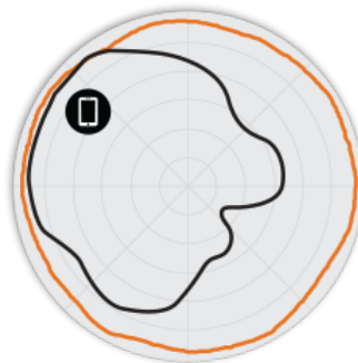
Figure 3. R710 5GHz Azimuth Antenna Patterns
