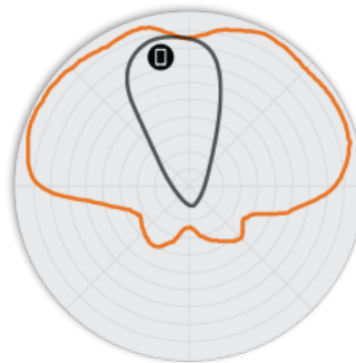
Figure 4. R710 2.4GHz Elevation Antenna Patterns
